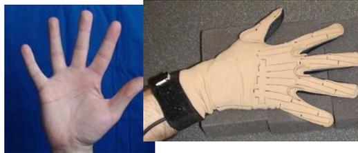
Alternate between the 'Flat B' and '5' handshapes, and modify the **gain** values of the four **abduction** joints. The goal is for the degree-of-arc of the human's movement to match the degree-of-arc of the on-screen hand.
